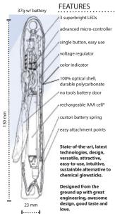
**Bright:** 3 regulated ultrabright LEDs provide maximum brightness for entire battery life.
